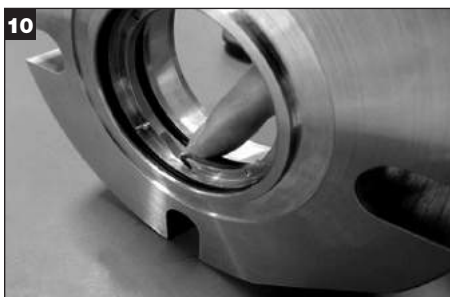
Remove both O-Rings from gland assembly and discard.
