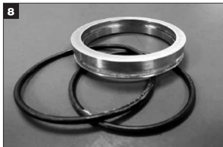
Remove two spacer O-Rings and discard.
