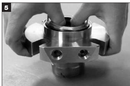
5 Separate gland assembly from sleeve assembly.
