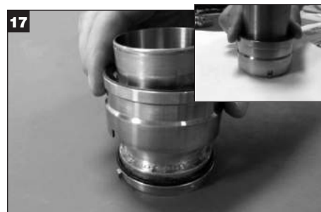
Slide rotary holder assembly over sleeve. Align slot in rotary holder assembly with lug in sleeve and compress.
