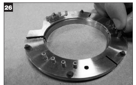
Apply a thin film of grease to one end of each spring and install springs in the lock ring.
