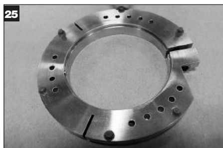
Install centering pins in lock ring.
