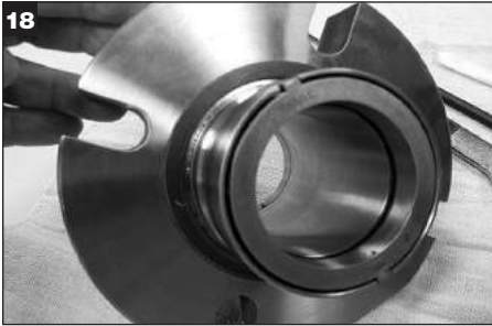
Remove backing and install gasket on clean surface of gland assembly.
