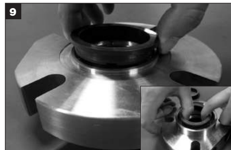
Remove both inboard stationary seal rings from gland assembly and discard.
