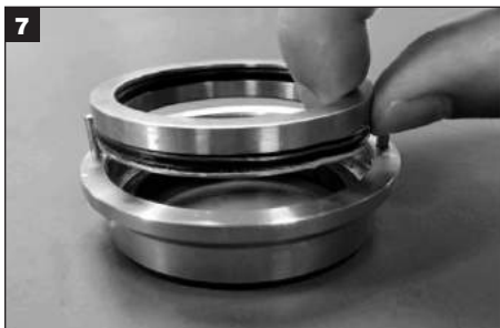
Separate spacer from outboard rotary seal ring assembly. Discard rotary seal assembly.
