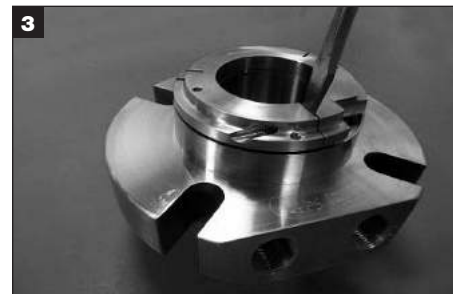
3 Using a leverage device, carefully disengage lock ring from sleeve.
