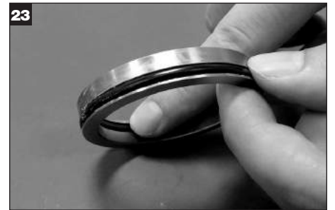
Apply a thin film of grease to the adapter O-Rings (2x) and install into the adapter O-Ring grooves.
