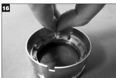
Apply a thin film of grease to one end of each spring and install springs in the inboard rotary assembly.
