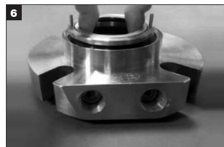
6 Remove outboard rotary seal ring assembly from gland.
