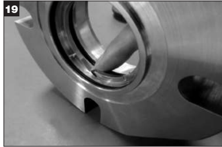
Apply a thin film of grease to the stationary O-Rings (2x) and install into the gland O-Ring grooves.
