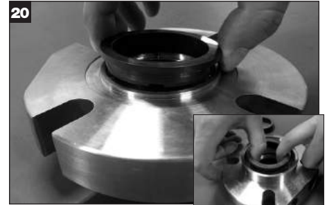
Apply grease to outside diameter of stationary seal faces. Align two slots in stationary seal face with two pins in gland and install stationary seal face. Wipe both seal faces with a clean dry cloth.
