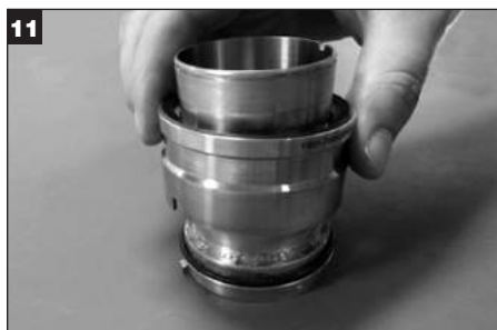
Remove the inboard rotary assembly and discard (including springs and O-Ring).
