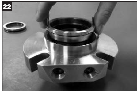
Wipe outboard rotary face with a clean dry cloth. Slide the outboard rotary assembly over the sleeve, ensuring the face mates with the outboard stationary seal face.
