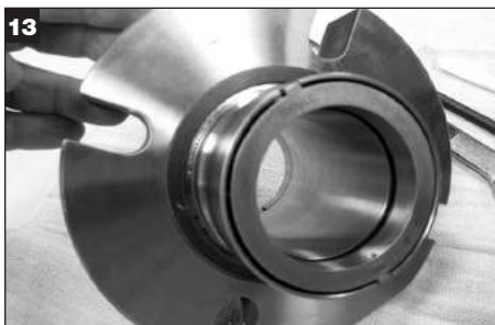
Remove gasket from gland assembly and discard.
